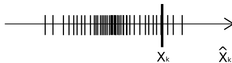
Figure 3.3: Problem of the rms analogy criterion. The small bars represent the historical data \hat{X}_k and the large bar the current value of X_k . It is clear that in this example more analog \hat{X}_k smaller X_k than greater X_k are found
